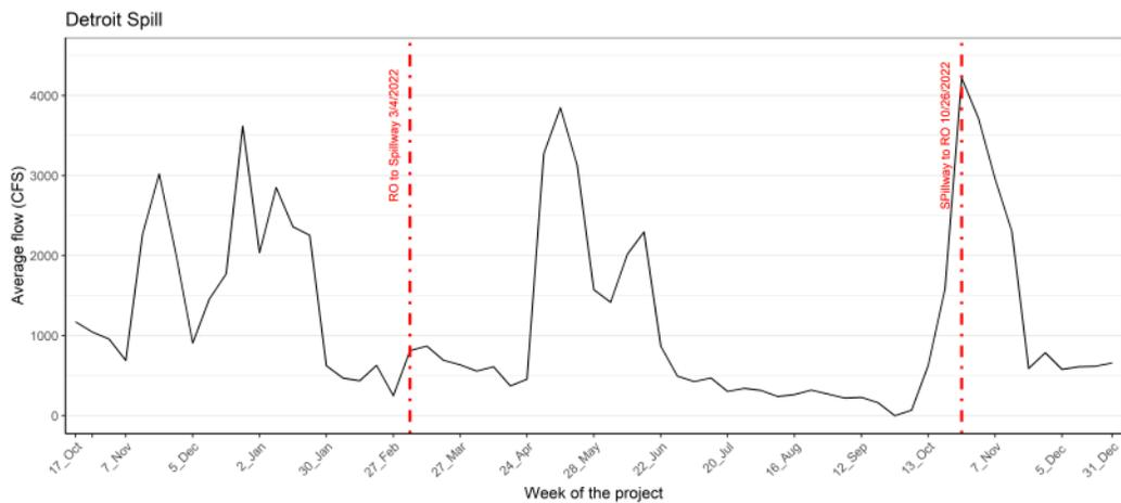
**Figure 4. Detroit spill operations from the initiation of sampling at Big Cliff through 2022.**
